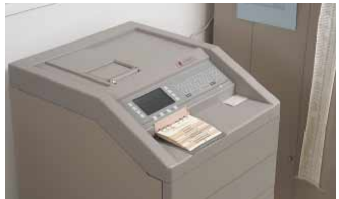
Figure 29-6 Computer-controlled Dispensing System
